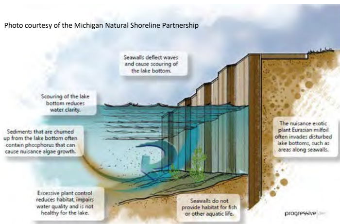
Figure 10. Illustration of wave action against a seawall.
