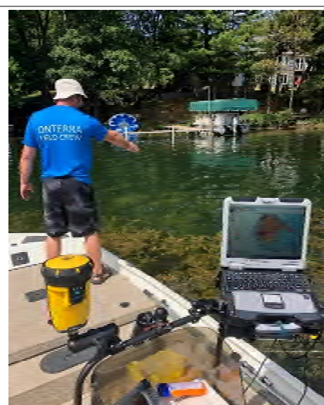
Photograph 3.4-10. EWM mapping survey on a Waushara County, WI lake. Photograph credit Onterra.
